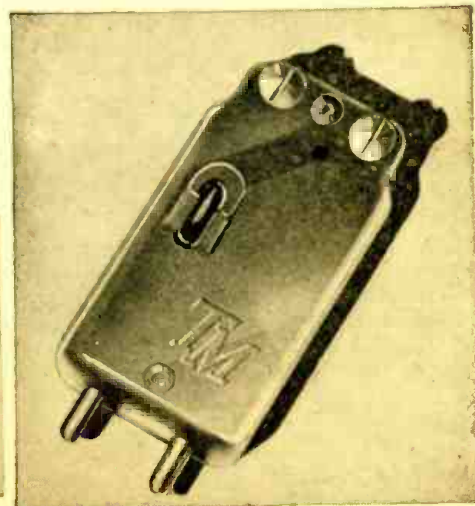
Photo B—Magnetostriction pickup in its case.
