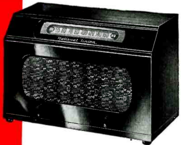
PRESENTATION MODEL No. G619. 6 Tubes. AC-DC. Tuned R.F. Stage. Superheterodyne Circuit. Loop Aerial. Automatic Volume Control. Illuminated Slide-Rule Dial. Standard American Broadcasts. Mahogany Veneer All-Wood Table Cabinet, 13" x 8 \frac{3}{4} " x 6 \frac{1}{2} ".
