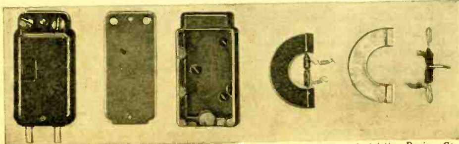
Photo A—Exploded view of the pickup. The important working parts are shown at right.
